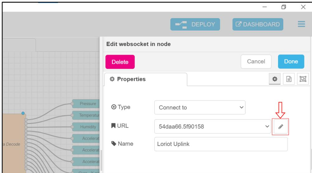
4. In this window, we must insert the URL. If the Loriot server is used, then the link must be taken from [2.4 Loriot Uplink](#). After inserting the URL, click on **Update**. This action is illustrated in Figure 67.
