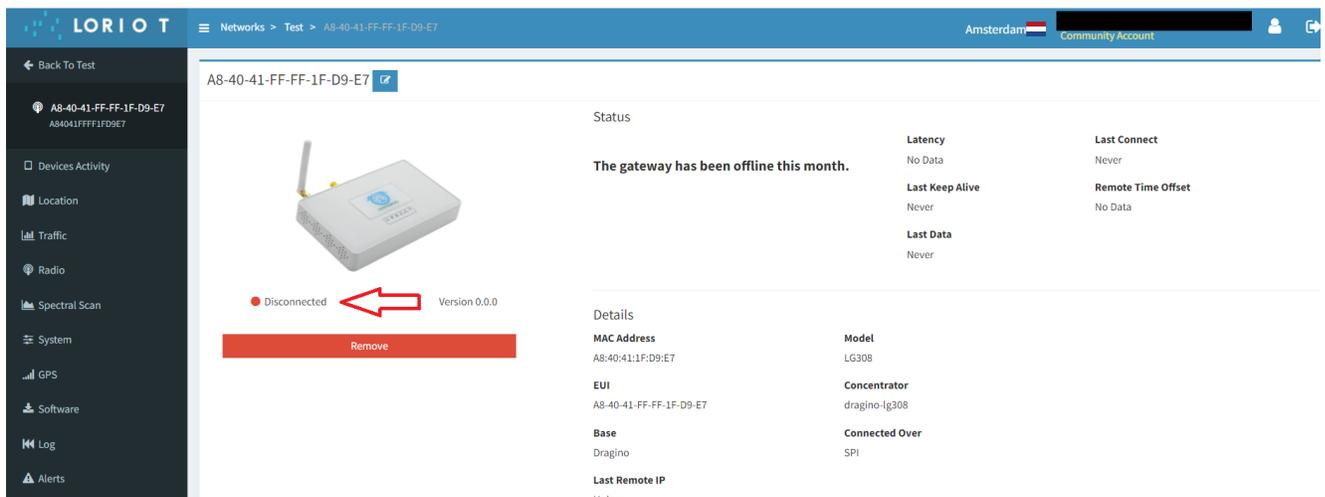
6. To speed up the procedure for connecting the gateway to the server, you need to reboot the gateway. Need to refresh the page and wait until the gateway status changes to connected (Figure 17).
