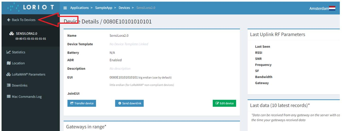
6. In the **Devices** tab, you can view the addition of a device. When the added device connects to the server then we should see the value: **RSSI, SNR, devSNR, SF and BAT**, for example, in Figure 23.
