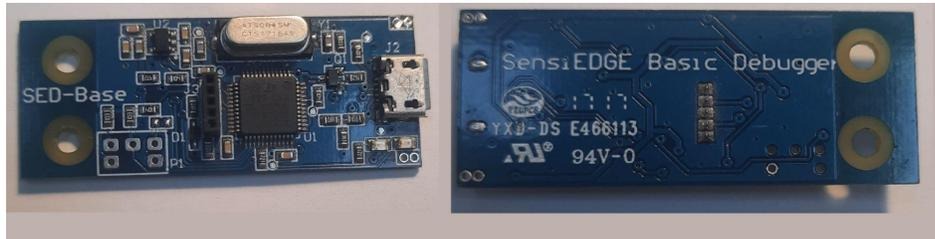
2. Connect the SensiLoRa 2.0 to the programmer SensiEdge Basic Debugger (Figure 75) and then connect the USB to the programmer.
