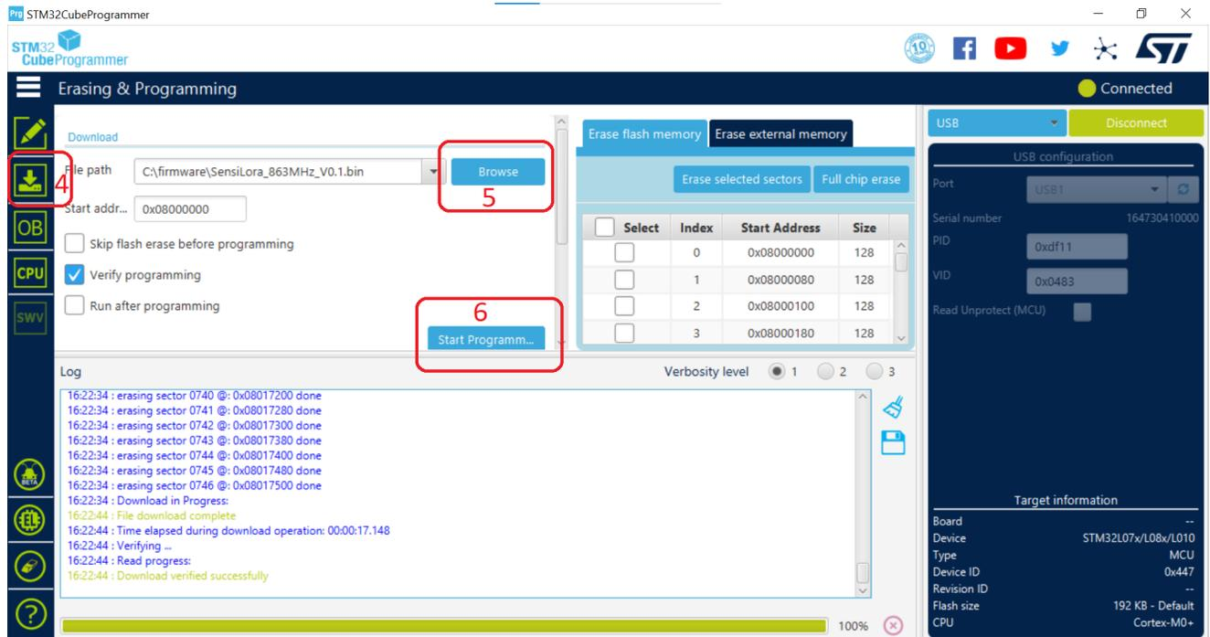
5. After successfully loading the firmware, we should see the message Download verified successfully (Figure 83).
