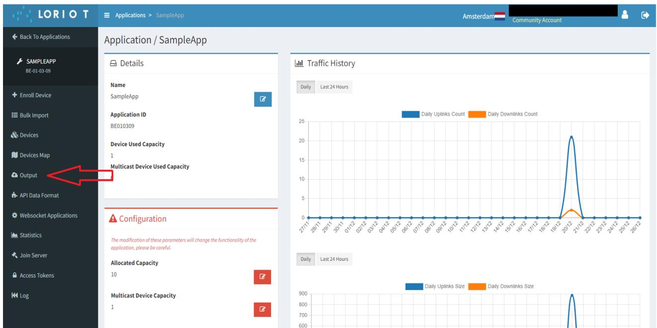
2. Data output link. Example: Use the **Target URL Template**, for example, Stm32CubeMonitor (Figure 25).
