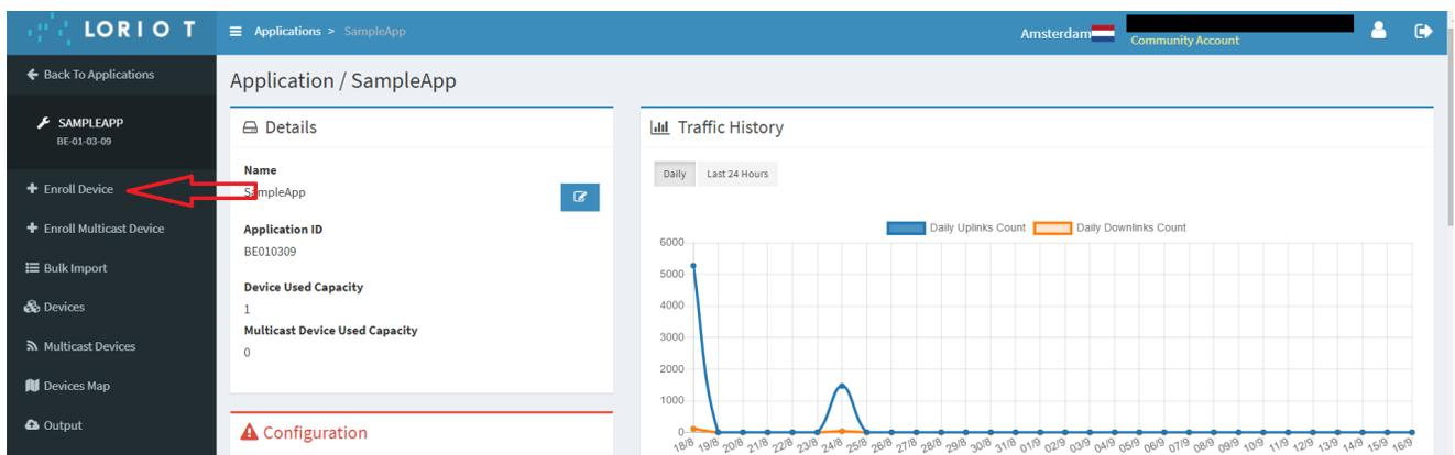
4. In the tab Enroll Device, enter any Name in **Title** (step 1), then enter **Application key** (step 4), **Device EUI** (step 2) and **Join Eui** (step 3), (this keys can be found using the SensiConfigurator program, download: [Ссылка на программу](#) . Use [Getting Started SensiConfigurator](#) document section [3.2 Device Information](#)). Click **Enroll** (step 5) (Figure 21).
