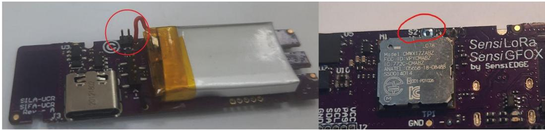
2. When holding down button S2 connect the cable USB Type-c (Figure 80) and after a couple of seconds we release the button with this combination, and the board enters the programming mode.
